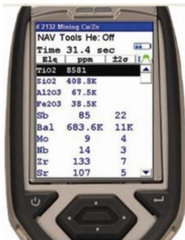
Figure 4: Elemental content from a rock (in ppm) recorded by a portable XRF instrument
