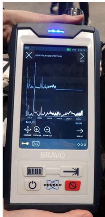
Figure 5: Bruker Bravo handheld Raman spectrometer as exhibited at the Perth Gem and Mineral Show (PGMS) in October 2021
