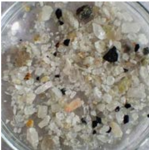
(A) Image shows a sample of coarse grains from the ball mill in a 3 cm diameter petri-dish. Spodumene is the dominant mineral, typically white or colourless and transparent the cleavages result in prismatic shaped grains. Dark fragments of almost-opaque green amphibole and rare grains of white mica, feldspar and quartz are all present in the sample.
