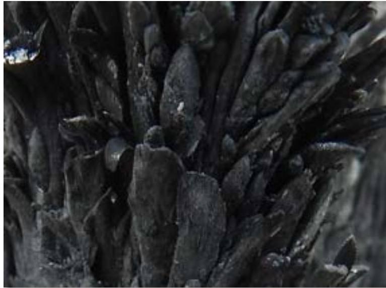
Figure 1. Crystalline silicon, manufactured; field of view is about 1 cm across
