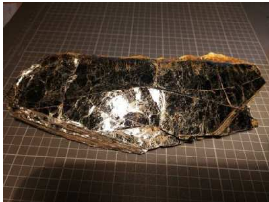
Biotite book – Mukinbudin Quarry – squares are 1cm x 1cm (Picture by Rob Walker)
