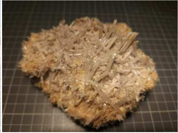
Lake Brown Gypsum – squares are 1cm x 1cm (Picture by Rob Walker)
