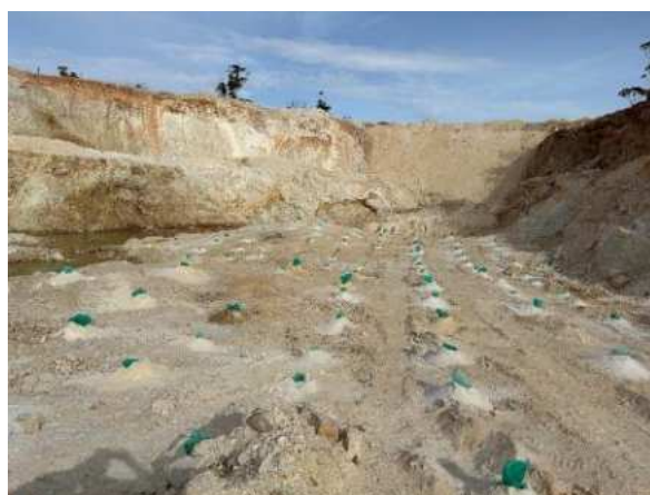
Blast pattern ready for charging (soapstone in brown on lower pit wall) - Potts Rd Quarry
