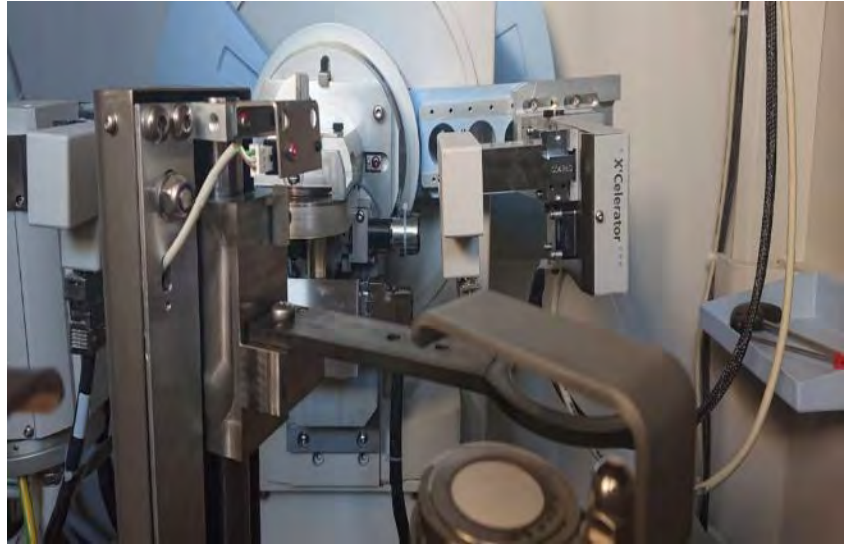
Internal mechanics of an x-ray diffractometer
