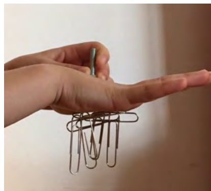
The magnetic field of this N52 neodymium magnet can pass through biological tissues
