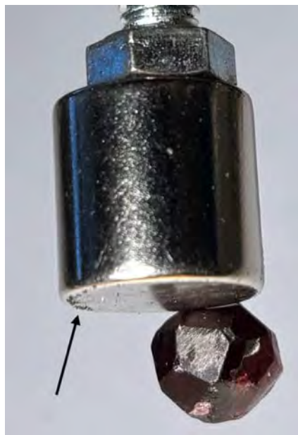
Two small neodymium magnets (8x3 mm) shattered upon rapid impact with a large 12x12 mm magnet.
